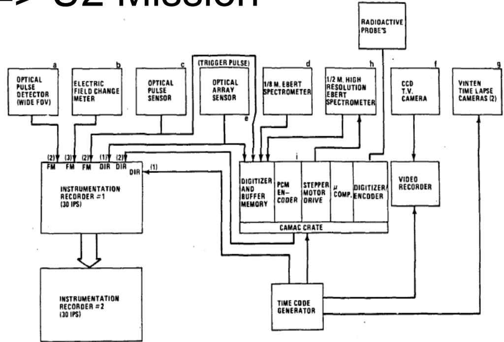
Fig. 1. Block diagram of U-2 aircraft lightning instrumentation.
